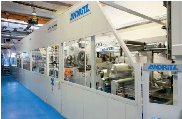
Spunlace pilot line at the technical center in Montbonnot, France
